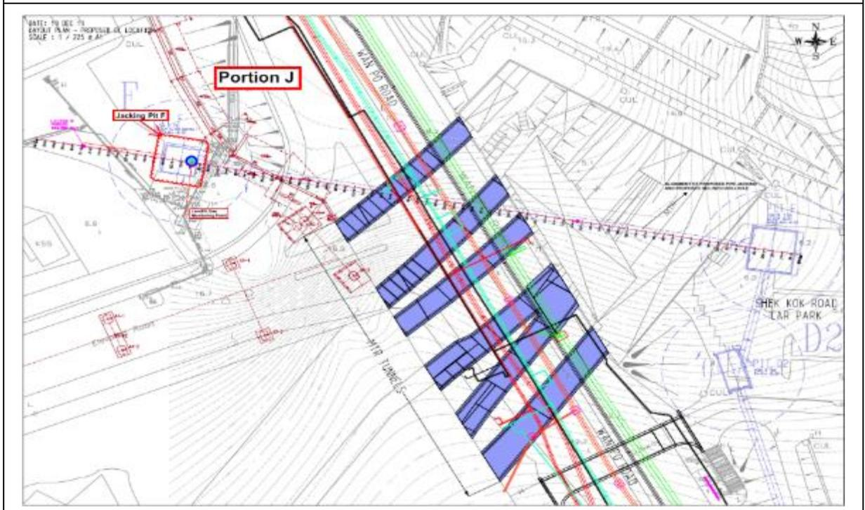
**Figure 4.9 Monitoring Location - Jacking Pit F**
